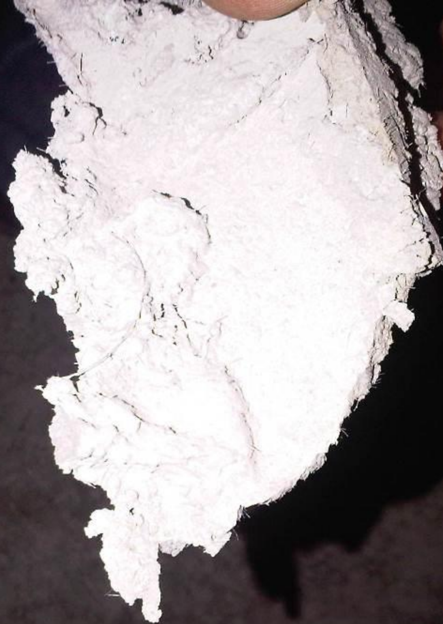
Asbestos cement/Hard coating on eg. Pipes(3)
